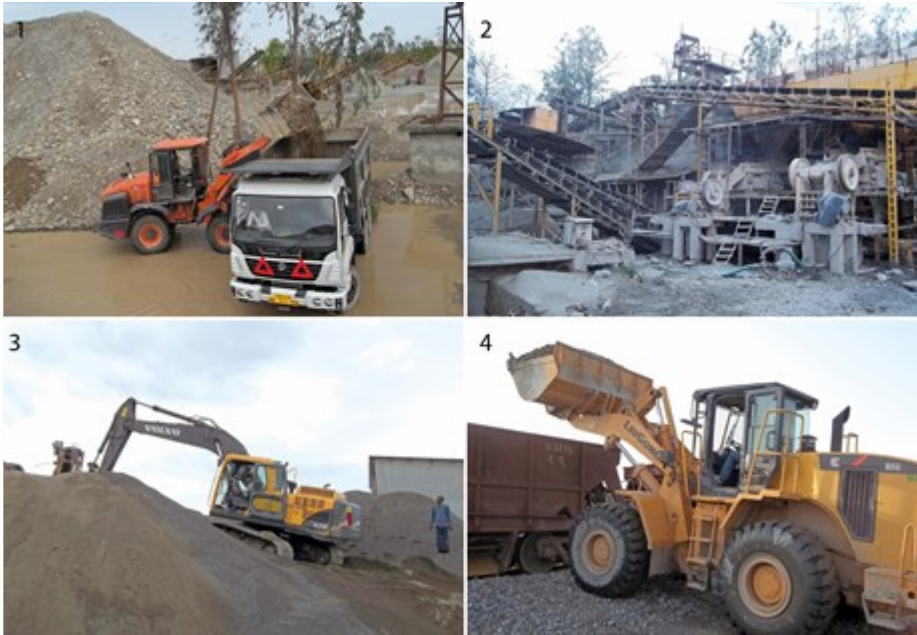
1. A Telcon Hitachi PML 3034 wheeled loader loading river bed materials on a new Ashok Leyland U-2516 tipper truck; 2. Jaw crushers in operation at LSC Infratech's Haldwani plant; 3. A Volvo EC 210 21tonne excavator loading crushed sand at Ajitpur plant; 4. A LiuGong CLG 856 5 wheeled loader loading crushed aggregates from one of LSC Infratech's quarries into a container ahead of being transported to upcoming railway projects in north and other parts of India
