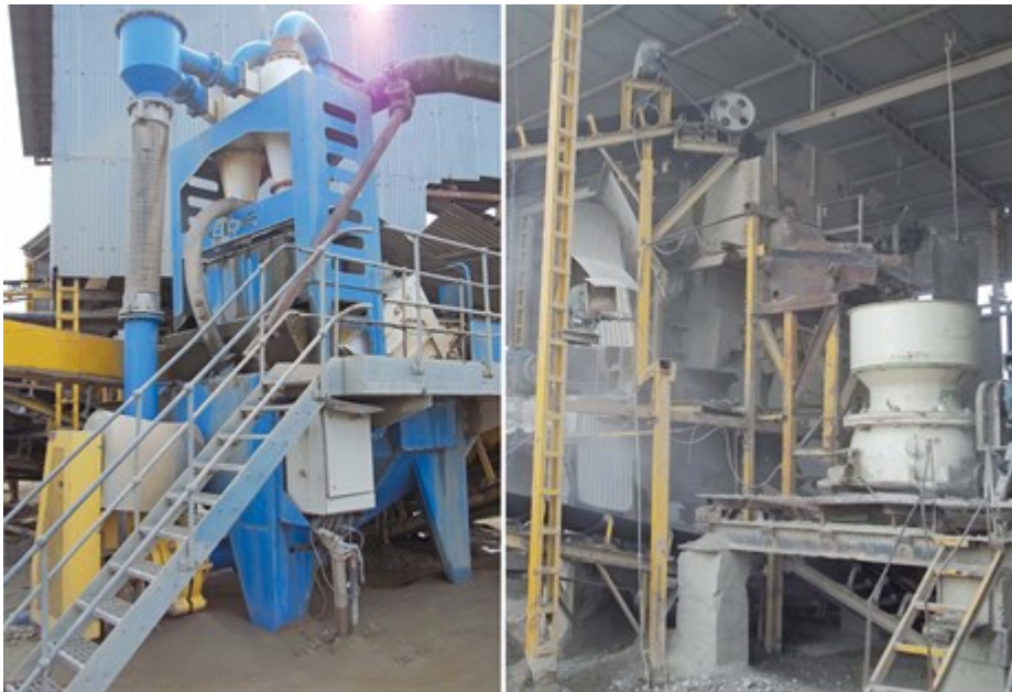
LEFT: CDE Asia B series sand washing plant at Ajitpur plant; RIGHT: The 220 tonnes/hour cone crusher from Propel Industries is well used at Ajitpur plant
