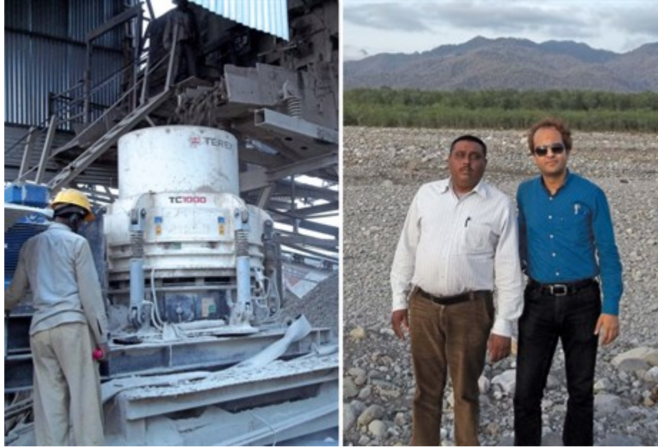
LEFT: A TC 1000 150tonnes/hour Terex MPS cone crusher at Haldwani plant; RIGHT: Article author Partha Pratim Basistha (right) at LSC Infratech's river bed boulder source in Uttarkhand with Sushil Chauhan, head of operations & maintenance at LSC Infratech
